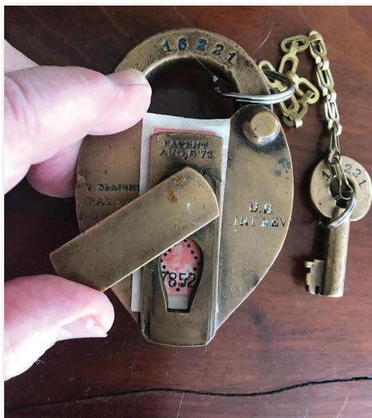
Figure 1. (Above left & right) The Slight lock that used intaglio printed paper lock seals supplied by the Bureau of Engraving & Printing.
