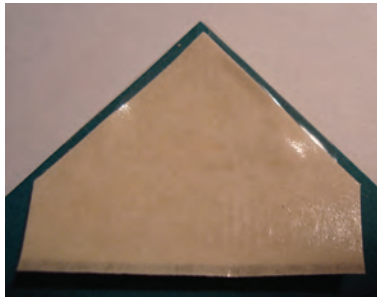
Figure 2a: Original corner – shown from back to illustrate clear edge (about 1mm wide)
